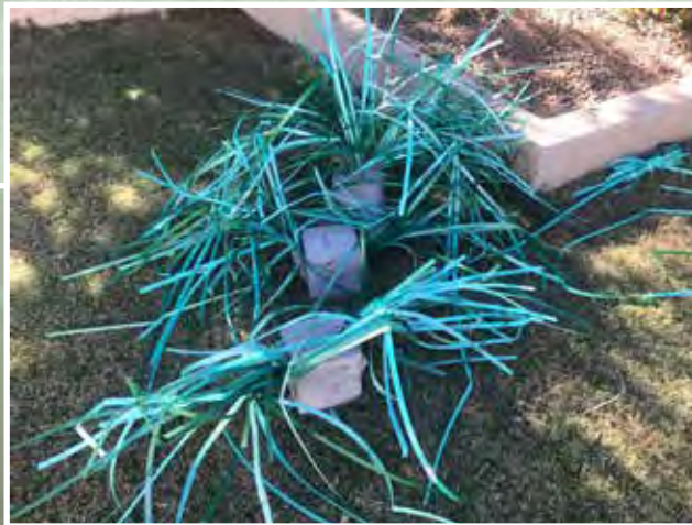
Polyester strapping is secured within concrete block to add weight
