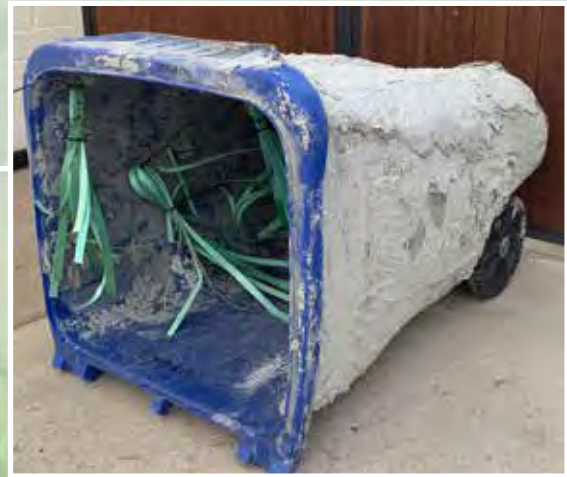
Strapping dangles from recycle bin to simulate plant roots
